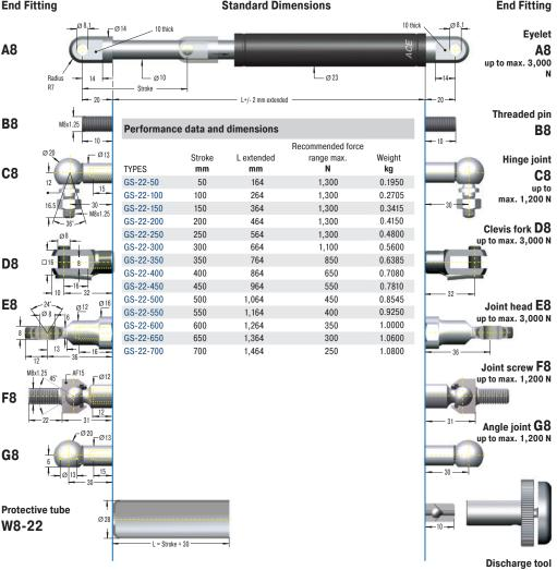
The end fittings can be combined in any manner and must be secured against twisting by the customer, if necessary. See mounting accessories.
