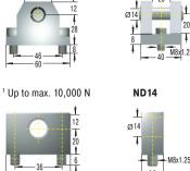
1 Note! Max, static load in N: note force increase when pushing in (progression). Higher load possible on request.
