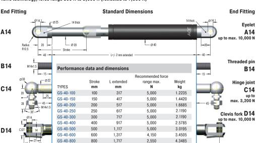
Only on request: This gas spring has to comply with the Pressure Equipment Directive (PED). A check of the application is necessary in individual cases. Please contact our technical service
