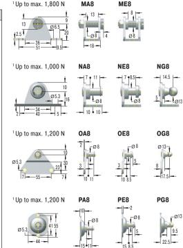
1 Note! Max. static load in N; note force increase when pushing in (progression). Higher load possible on request.
