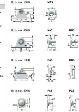
1 Note! Max. static load in N; note force increase when pushing in (progression). Higher load possible on request.
