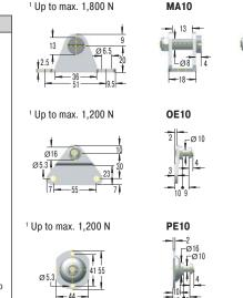
1 Note! Max. static load in N; note force increase when pushing in (progression). Higher load possible on request.
