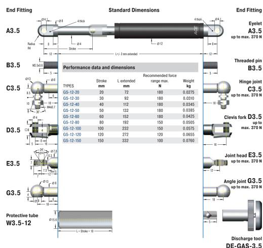
The end fittings can be combined in any manner and must be secured against twisting by the customer, if necessary. See mounting accessories.
