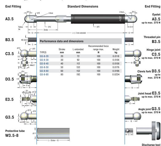
The end fittings can be combined in any manner and must be secured against twisting by the customer, if necessary. See mounting accessories.
