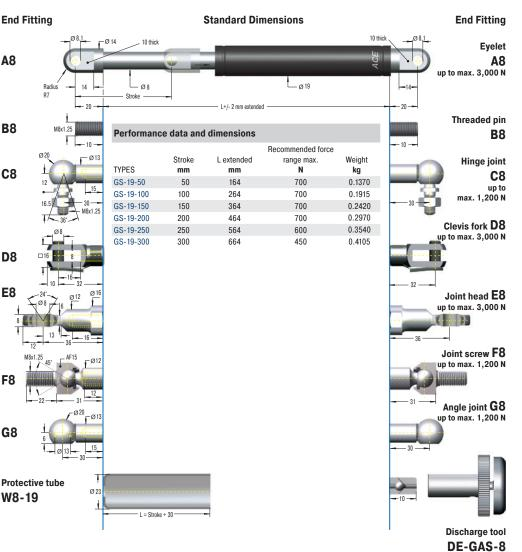
The end fittings can be combined in any manner and must be secured against twisting by the customer, if necessary. See mounting accessories.
